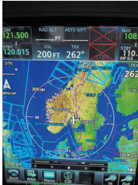
FIGURE 2: AVIONICS SECURITY LABORATORY UNDER GPS SPOOFING. THE GARMIN SYSTEM SHOWS ITS GPS POSITION IN SCANDINAVIA DESPITE BEING LOCATED IN SWITZERLAND
