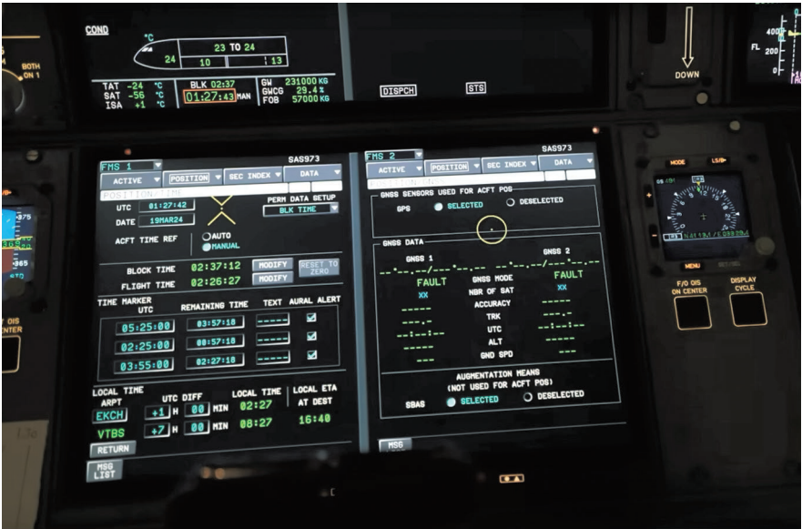
FIGURE 1: GPS JAMMING AS SEEN ON AN SAS AIRBUS A350 FROM COPENHAGEN TO BANGKOK. INTERFERENCE WAS REPORTED FROM POLAND TO THE PERSIAN GULF [15], [16]
