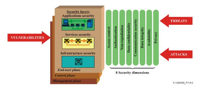
Figure 7-4.2 – Security planes reflect the different types of network activities
