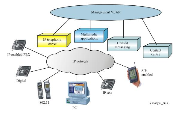
**Figure III.2 – Securing IP telephony**
