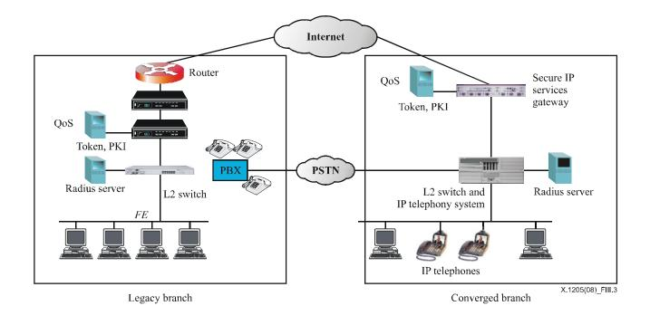
**Figure III.3 – Securing remote office**
