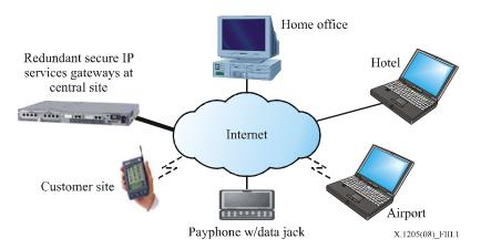
Figure III.1 – Securing remote access
