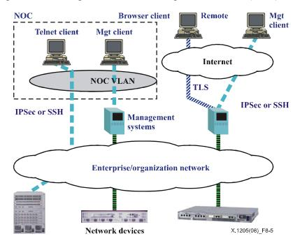
Figure 8-5 – Reference model for securing management
