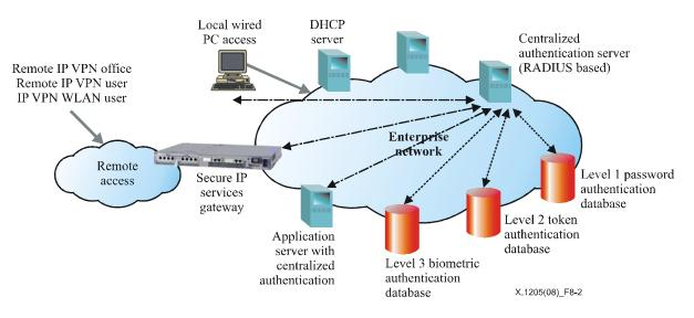
Figure 8-2 – Secure authentication and authorization reference model
