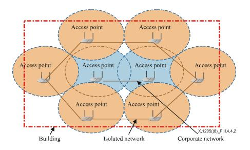
Figure III.4.4.2 – Sentry APs for perimeter security
